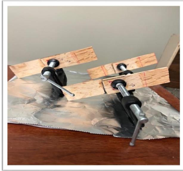
**Figure 19:** Manual clamping method
