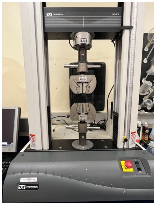
**Figure 11:** Digital image of the lap shear strength instrument used in this research
