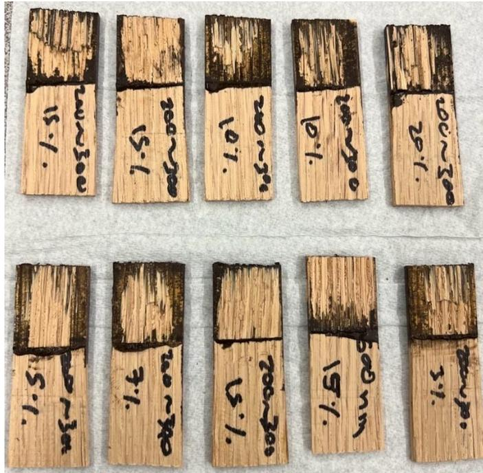
**Figure 21:** Substrate failure observed in specimens
