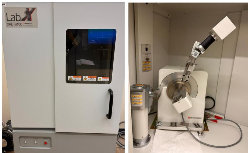
**Figure 2.3:** Digital images of Shimadzu X-ray diffractometer used in this research.
