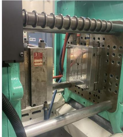
**Figure 20.** Test bar mold within the Arburg.
