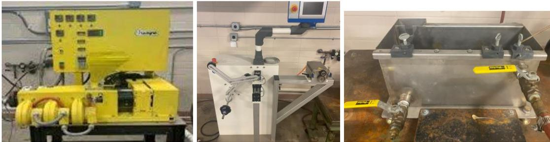
**Figure 14.** Wayne Yellowjacket single-screw extruder (left), Brabender puller/winder (center), and water bath for filament cooling (right).
