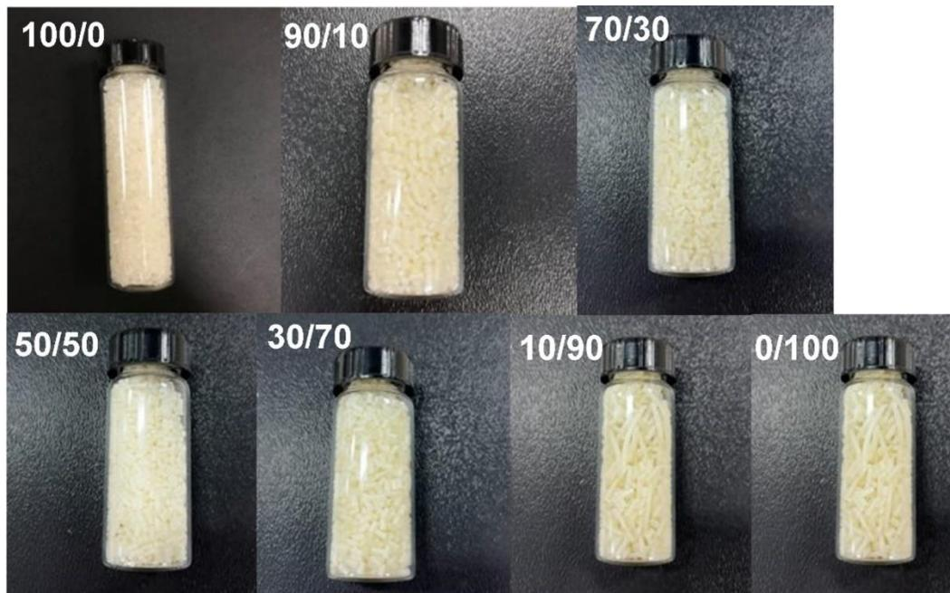
**Figure 35.** Appearance of 100/0, 90/10, 70/30, 50/50, 30/70, 10/90, and 0/100 twin-screw pellets.
