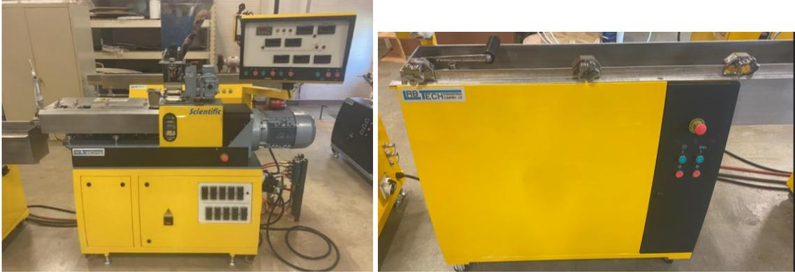
**Figure 16.** LabTech twin-screw extruder (left) and LabTech water bath (right).
