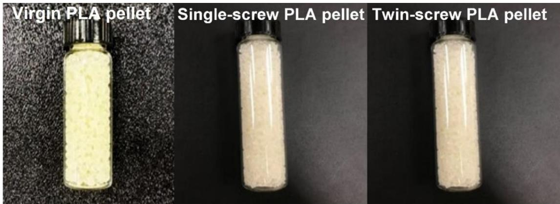
**Figure 24.** Appearance of virgin, single-screw, and twin-screw PLA pellets.
