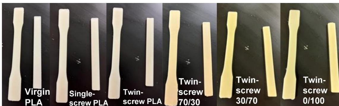
**Figure 39.** Appearance of virgin PLA, single-screw PLA, twin-screw PLA, twin-screw 70/30, twin-screw 30/70, and twin-screw 0/100 injection-molded test bars.
