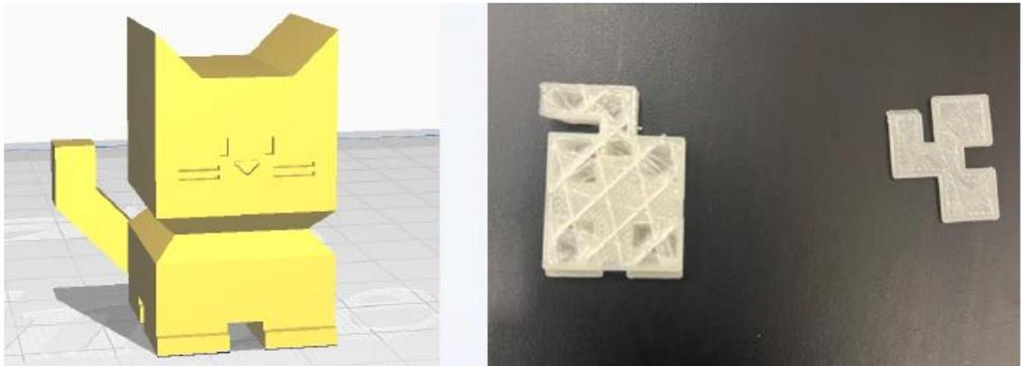
**Figure 41.** Proposed 3D printed part design (left) and actual printed part made with 100/0 PLA filament processed by twin-screw extrusion (right).
