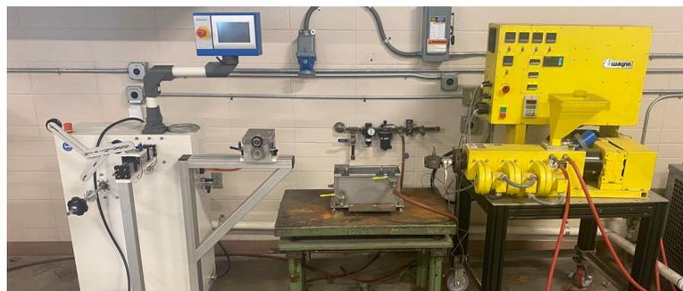
**Figure 15.** Complete single-screw extrusion line.
