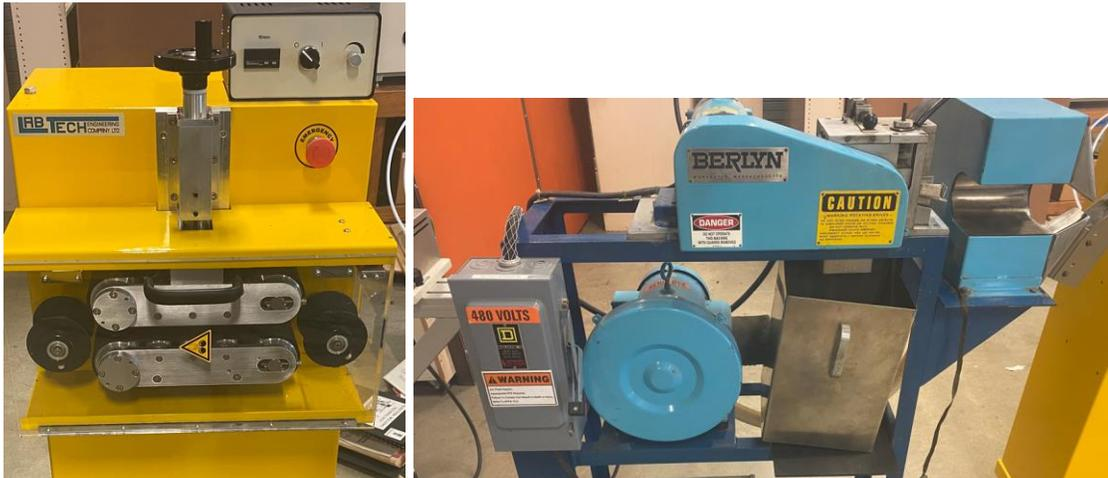
**Figure 17.** Labtech puller (left) and Berlyn material grinder (right).
