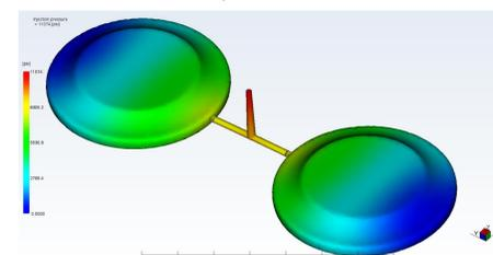
Figure 4. MoldFlow Injection Pressure for Frisbee Parts.
