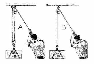
Which man must pull harder to lift the weight?
