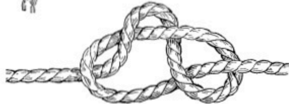
METHOD OF ATTACHING PENDENT CORDS
